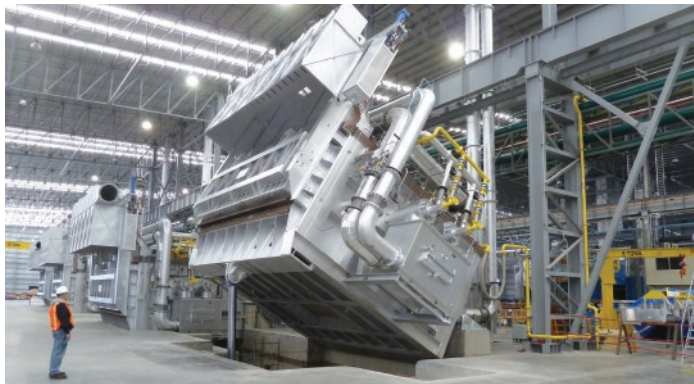
Conclusion of the tilting test for a series of GNA 40 t melting furnaces.
